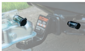
Watertight dust caps prevent internal corrosion
