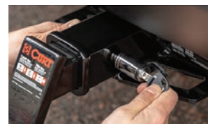
Easy-to-operate, 1/4-turn lock activation
