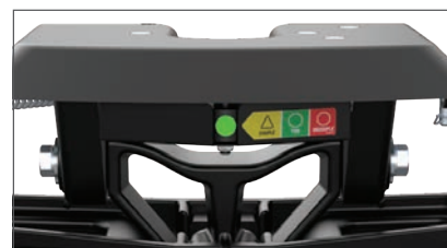
Three-position coupling indicator clearly shows coupling status
