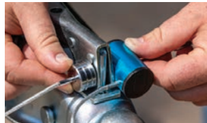
Coupler lock can also be used while towing to secure the trailer
