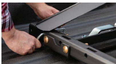
Industry-standard rails accept most 5th wheel legs and rollers
