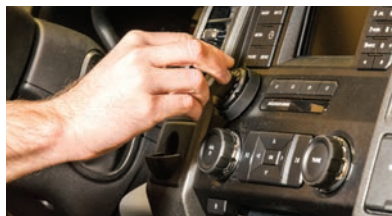
Clean, dash-mounted, OEM-style user interface with 10 tri-color LEDs
