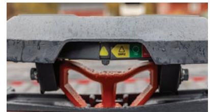
Three-position coupling indicator clearly shows coupling status
