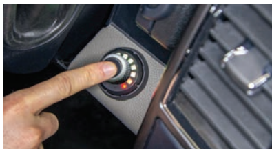
Controls all brake settings with a simple push-button rotary knob
