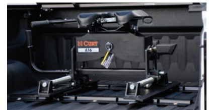
Uses wheels to bear the weight, instead of hollow rods like competition
