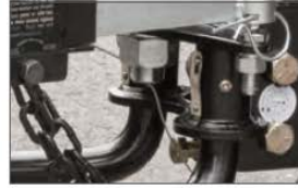
Easily-access grease zerk fittings
