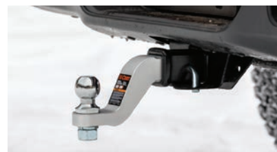
Constructed from solid aluminum to be lightweight and naturally rust-resistant
