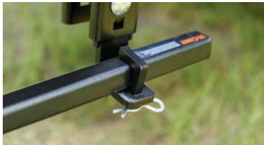
Two points of sway control use friction to keep trailer aligned
