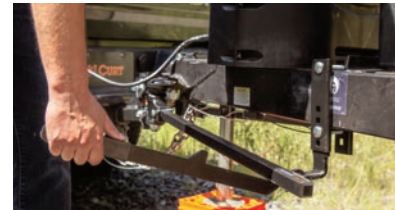
Adjustable brackets provide fixed support unlike spring bar chain models
